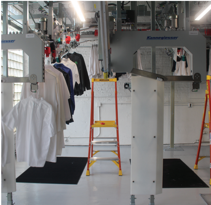
ABOVE: A view of the new garment sorter with its RF chipped red carrier hangers that enable the system’s antennae to read both the carrier and the garment chips and provide that information to the sorting system. Julia and Jim Buik stand beside the new sorter in a refurbished area of the 100-year-old plant.
